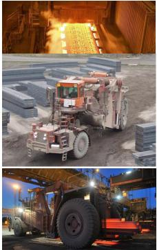
The goal of this master thesis is to model the heat transfer from the slabs to the slab carriers and do a proposition for at which cycle time or temperature limit the vehicle should be cooled down, and for how long, depending on the slab temperatures it has been exposed to.
